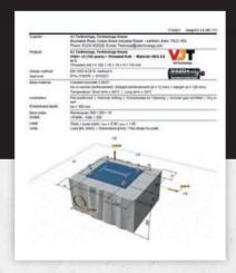
The calculation tab offers a print preview option and/or PDF which produces a results report. Anchor loads and potential modes of failure are detailed as well as installation information.
