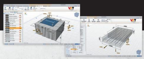
Live calculations change accordingly displaying product optimisation (design life of 50-100 years). Embedment depths are easily adjusted via a drop down menu whilst a series of tabs along the top allow the user to quickly make the amendments to concrete strength, geometry, properties and loads required.
